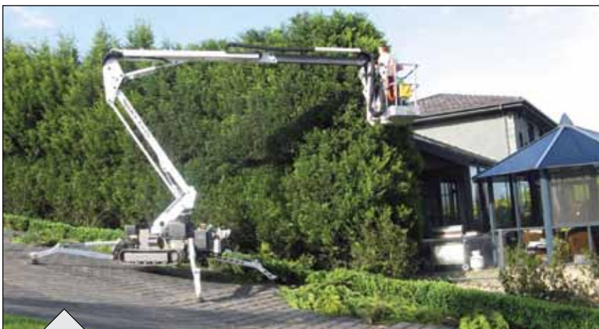
The extra-long travel stabilizer legs on the 1890 makes it the first choice for working on sloping sites.
