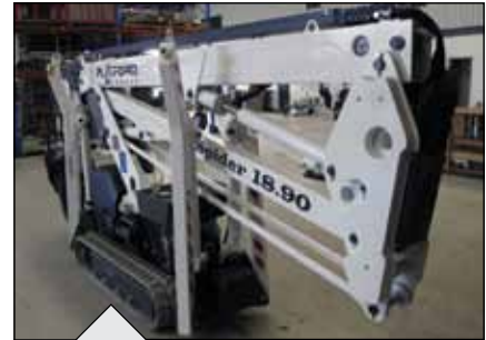
With the tracks retracted, the 18.90 has an incredible stowed dimension of only 792 x 1951 mm which allows it to drive through a domestic doorway!
