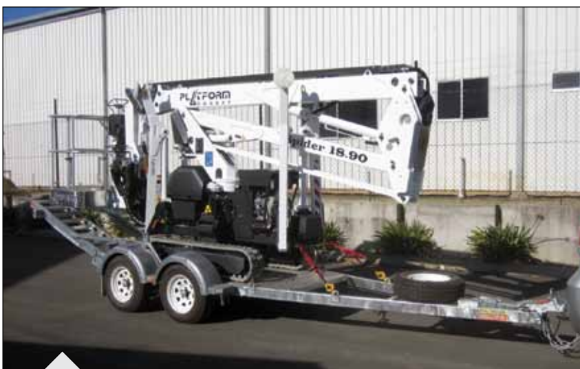
Weighing in at only 2.45 tonnes in weight, the 1890 is very easily transported on its strong gal steel trailer.
